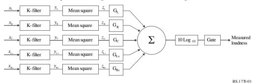
The first step of the algorithm applies a 2-stage pre-filtering<sup>1</sup> of the signal. The first stage of the pre-filtering accounts for the acoustic effects of the head, where the head is modelled as a rigid sphere. The response is shown in Fig. 2.
