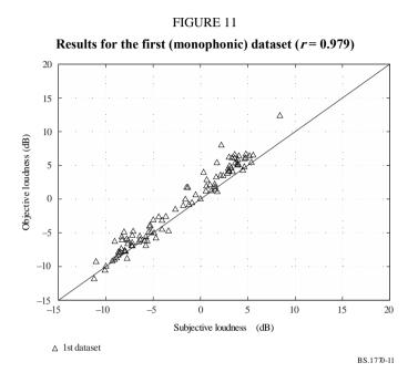
It can be seen from Fig. 11 that the proposed multichannel loudness algorithm performs very well at predicting the results from the first (monophonic) dataset. The correlation between the subjective loudness ratings and the objective loudness measure is r = 0.979.
