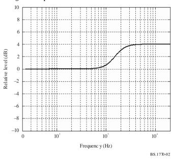
Stage 1 of the pre-filter is defined by the filter shown in Fig. 3 with the coefficients specified in Table 1.
