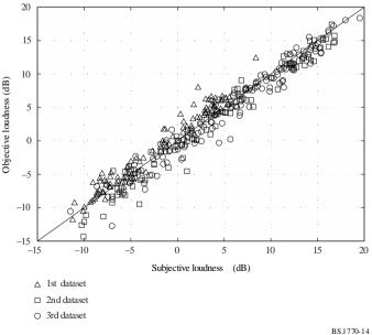
The results of this evaluation indicate that the multichannel loudness measurement algorithm, based on the Leg(RLB) loudness measure, performs very well over the 336 sequences of the subjective
